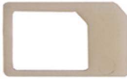
The micro-SIM carry board. Put the Micro-SIM card to the standard SIM card type carry board and plug into the system.
