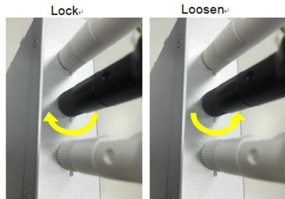
**For vibration environment,** it is still suggested you install the antenna at non-vibration or low vibration place and connect it by extended Radio cable antenna to the device.
