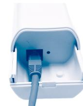
3. Slide the cover back to seal the bottom of JetWave 2450.
