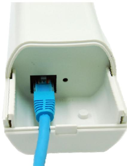
**Figure 4 Cable Connection**
