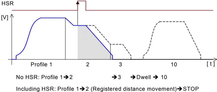
**Registration Move Distance (Common Parameter 24):** Specify the number of pulses from the axis should output when the High-Speed Registration input (above) turns on. Defaults to 10,000. This is a double-word floating point or integer value in the range 0 to +2,147,483,583.
