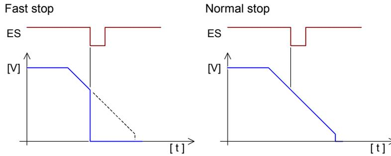
An error is generated when the Emergency Stop input goes off.
