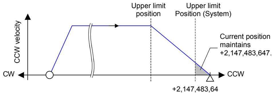
During Manual Mode operation when the Motion Type is Linear, if the target position exceeds this limit in the forward direction, the position error causes the axis to slow to a stop.
