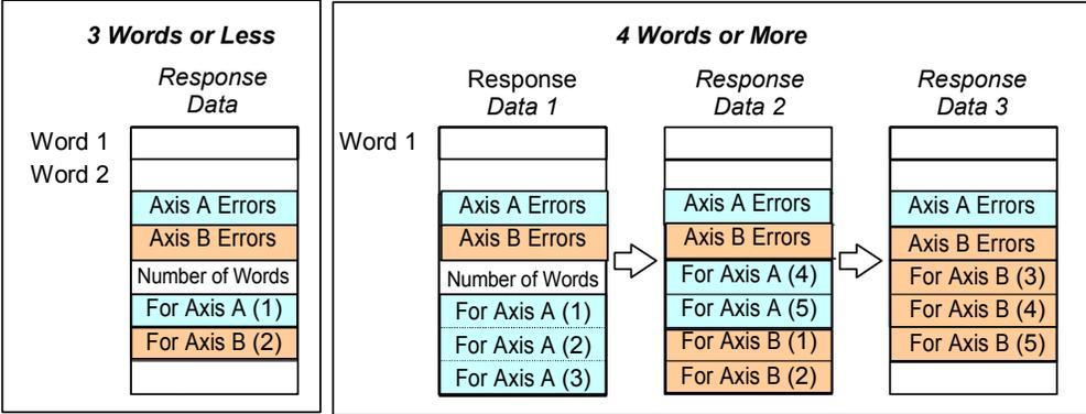
Input Status Data response to commands for reading parameters for which no axis is specified is shown below. Data is set in order from word 5. The number of words is specified in word 5 of the first handshake.
