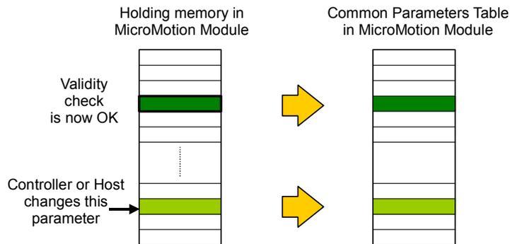
If setting up a Common Parameter fails, the operation cannot be executed until the error is cleared and a correct parameter is supplied.
