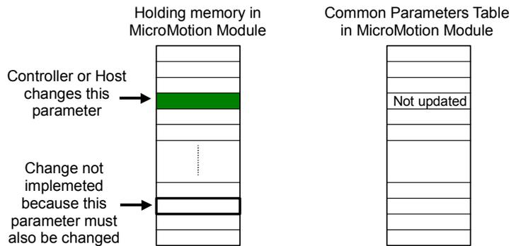
After the additional parameter change, the module again checks the validity of the change. If the subsequent parameter change makes the first parameter change valid, the module accepts both changed parameters and will use them. This procedure needs to be continued until there is no error.
