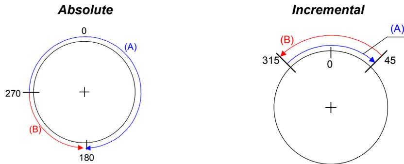
In Absolute + Incremental Positioning, if the Upper Position Limit is 0, the current position of the axis will never reach the Upper Position Limit.
