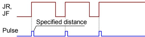
In Inching plus Jog mode, if the Jog Forward or Jog Reverse input is On, a pulse is output at the Initial Velocity that has been set up for Manual Mode. If Jog Forward or Jog Reverse remains on after 200ms, the pulse accelerates to the configured initial velocity at the configured acceleration rate. If the Jog Forward or Jog Reverse input is turned off, the pulse decelerates to the initial velocity at the specified deceleration rate, and stops.
