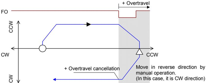
If an Overtravel input has been turned Off by the overtravel move, it remains Off until motion reverses back past the overtravel on position.
