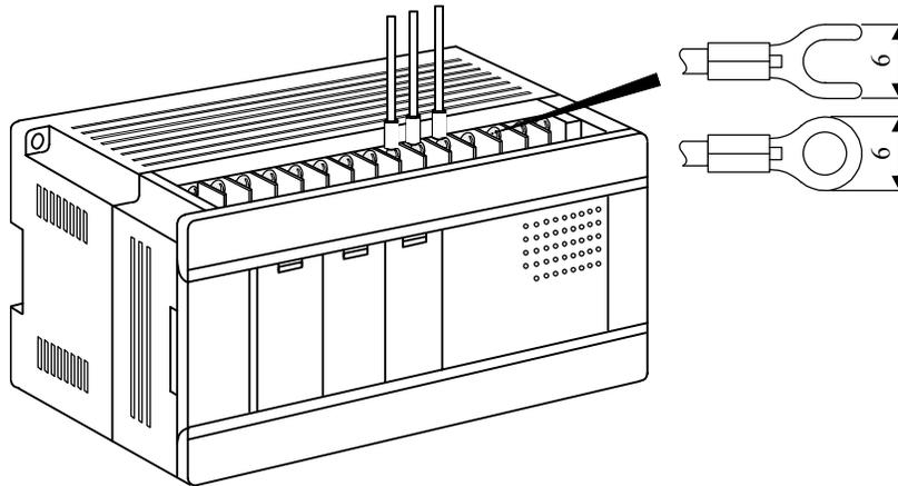
Use copper conductors rated for 75 °C (167 °F) for all wiring.
