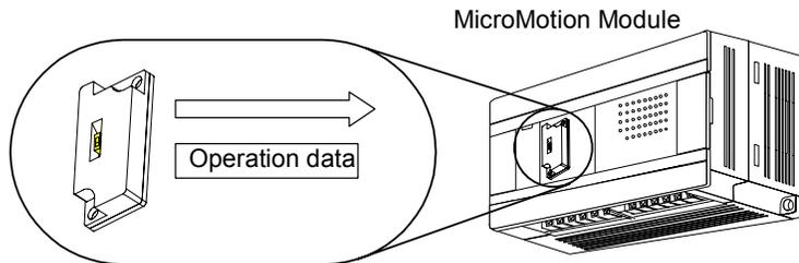
The ST2 LED keeps blinking while the data is being transferred from the Memory Pack. Wait until the ST2 LED stops blinking to do any further operations.
