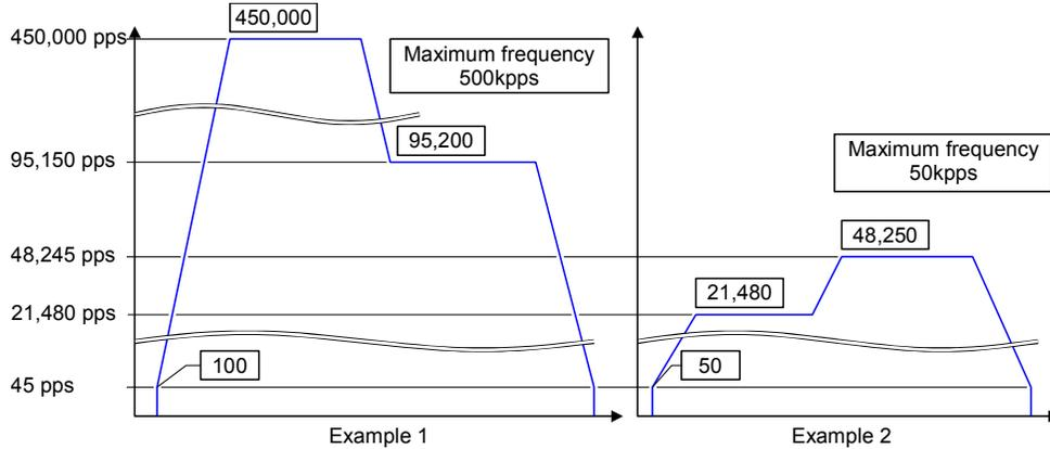
In example 1, the velocity units are 100 pps because the Velocity Limit is 500k pps (see the table on the previous page). Therefore, 95,150 pps would be adjusted to 95,200pps and 45 pps would be adjusted to 100 pps.
