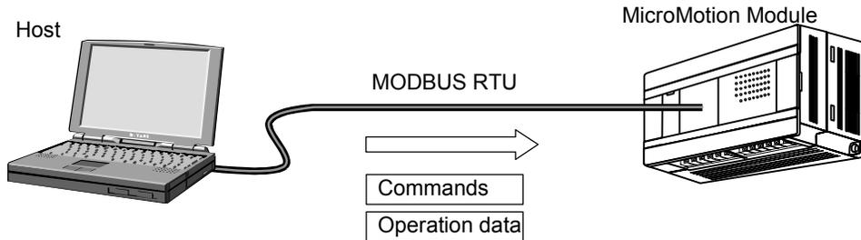
When the DIP switch 1 on the MicroMotion Module is Off (the default), the communication parameters are set to their defaults.
