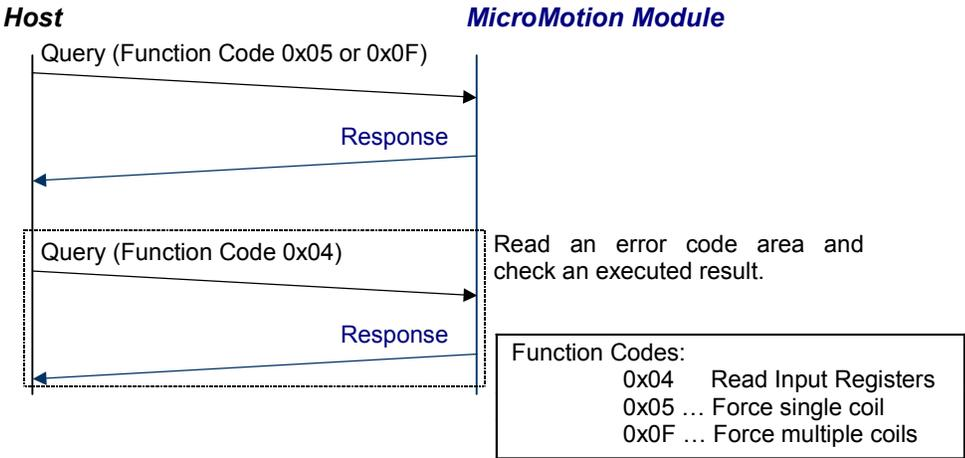
Coils for requests like start operation or stop operation are turned off by the system. Coils that stop a manual operation are *not* turned off automatically; they must be turned off by the user.
