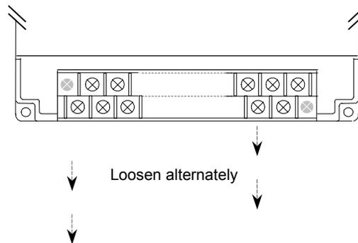
When re-installing terminal assemblies, be sure to place each one in the correct location to avoid miss-wiring the module. The terminal assemblies are not keyed or labeled.
