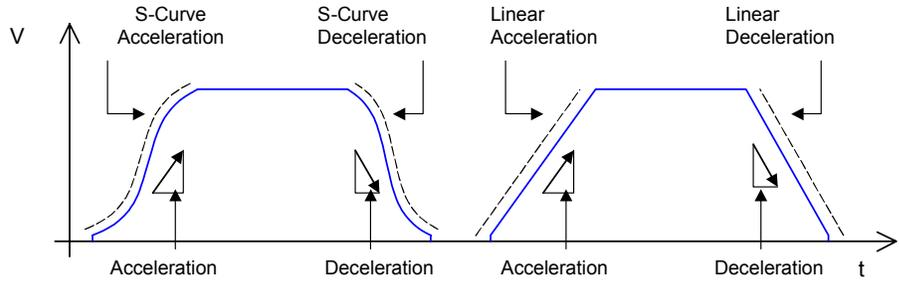
**Deceleration:** Set the Deceleration type to Linear or S-Curve.
