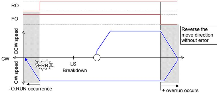
The Overrun (FO / RO) and Emergency Stop (ES) inputs can stop the pulse output. Whether these inputs cause a normal stop or a fast stop depends on their Common Parameter setting. If the move velocity is slow, a fast stop is always used.
