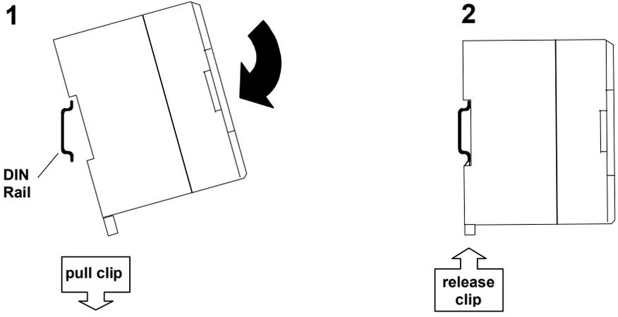
Secure the module by installing DIN rail brackets from both sides. (The module may shift on the DIN rail if it is not secured with mounting brackets.)
