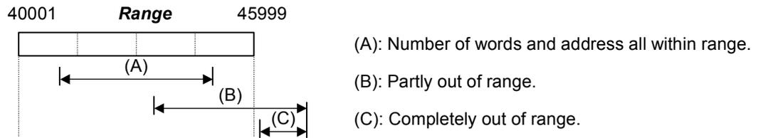
Holding Registers that are not currently being used are normally set to 0. If function code 0x06 or 0x10 writes data to an unassigned Holding Register, the module retains the value that is written. However, that does affect the operation of the module. Values in the Holding Registers do not control module operation until their corresponding coils are set to 1, as described previously.
