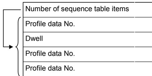
In the Sequence Table, each profile or dwell is represented as a number, which is the hexadecimal value equivalent to the bits in the profile or dwell. The format of the bits in the profile or dwell is shown on the next page.
