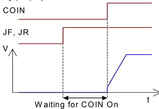
If COIN is Off at the start of the motion, an error is generated. Once the motion is in progress, the state of COIN is ignored.
