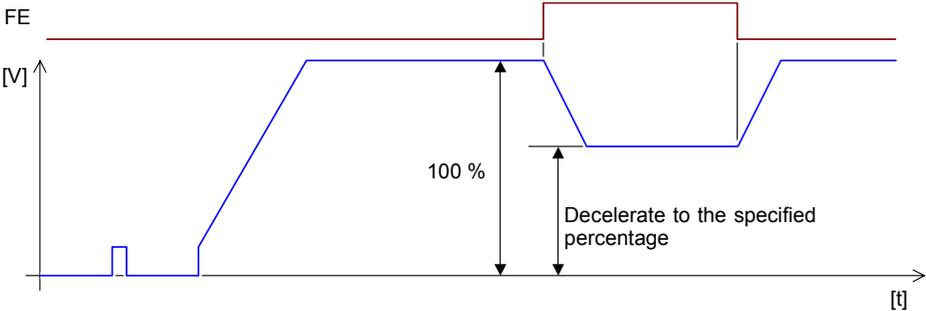
The rate of deceleration used for Feedrate Override can be specified from 1% to 100%, but the pulse will not slow down below the initial velocity, even if a slower speed is specified.
