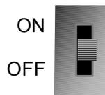
When the Write Protect switch on the Memory Pack is in the On position, it prevents writing data to the Memory Pack.
