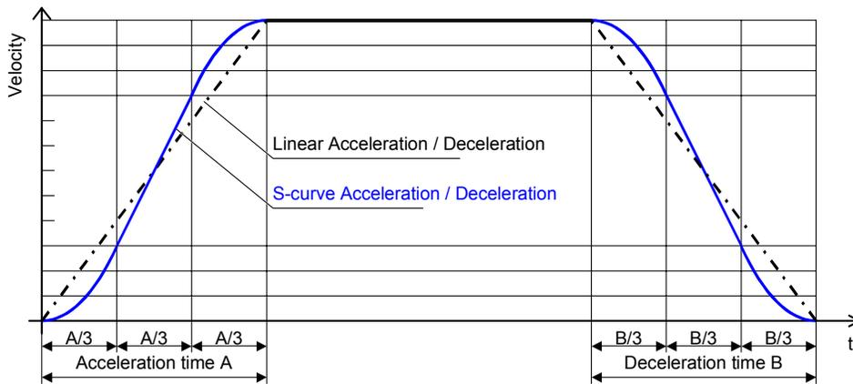
**Deceleration Type:** Set the deceleration for high-speed homing to Linear or S-Curve.
