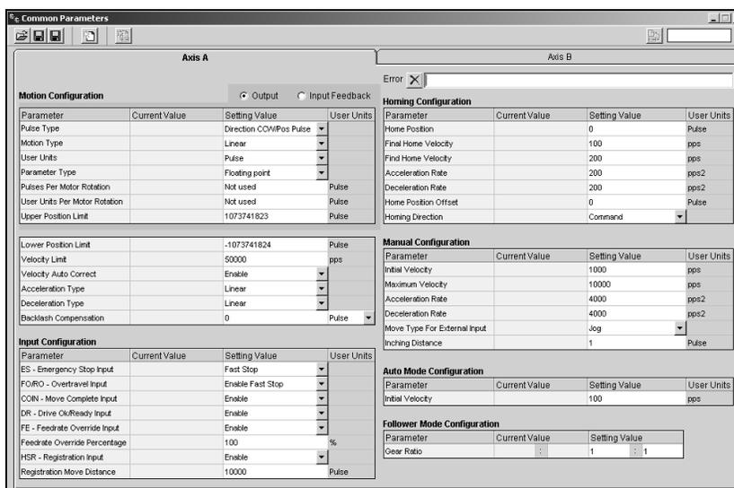
If the setup tool is communicating with a MicroMotion module, the current values are also displayed:
