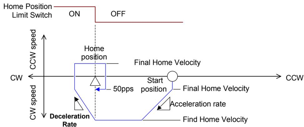
***If the Home Position Limit Switch was On at the start of High-Speed Homing [Off Edge]:***
