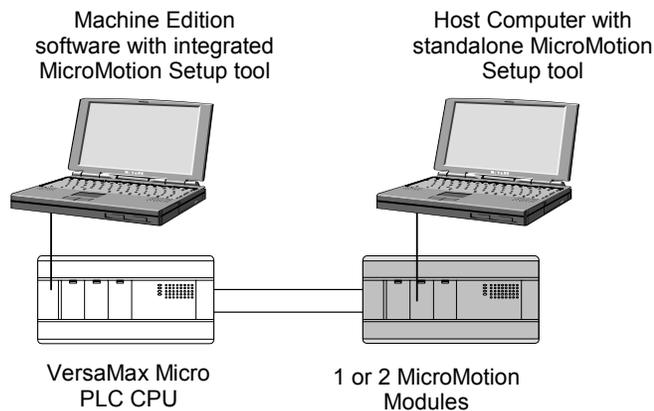
In addition to the monitoring and control provided by the user interface in the MicroMotion Setup Tool, motion operations can be set up, controlled, and monitored by the application program in the Micro PLC CPU using the module's assigned input and output status data as described in chapter 7. The host controller can also monitor and control motion operations using MODBUS RTU commands as described in chapters 8 and 9.
