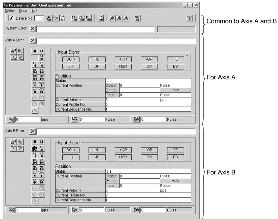
The Axis A and Axis B monitoring areas appear when the Setup Tool is in Online mode.
