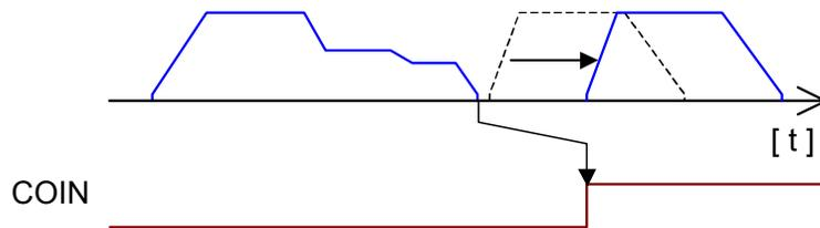
If a stop occurs because of an external input or Stop command, the MicroMotion Module completes the Stop processing before turning On the Move Complete input. The application logic in the CPU or host should check the Move Complete (COIN) input status. If the operation is restarted while the Move Complete input is still Off, an error occurs and the operation does not start.
