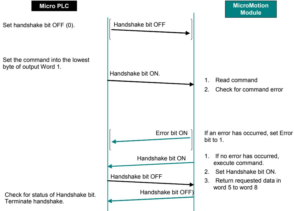
The read data is held while the handshake bit in the Output Control Data is On. If the handshake bit in the Output Control Data goes Off, data update is restarted using the same data format as before the Read command was executed.
