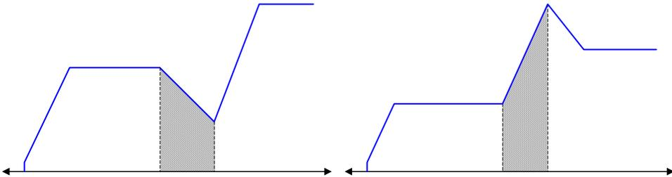
If the profile transitions directly from deceleration to acceleration, the velocity may drop suddenly.
