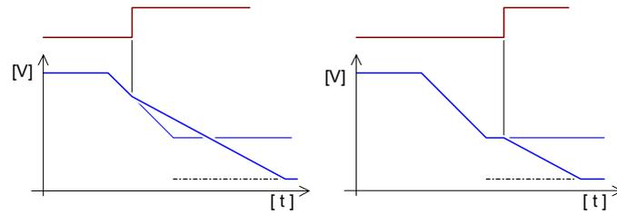
*FE Input OFF when Decelerating During Feedrate Override*
