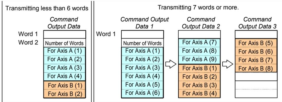
Output control data for transmitting of parameters for which no axis is specified is shown below. Data is set in order from word 2. The number of words is specified in word 2 of the first handshake.
