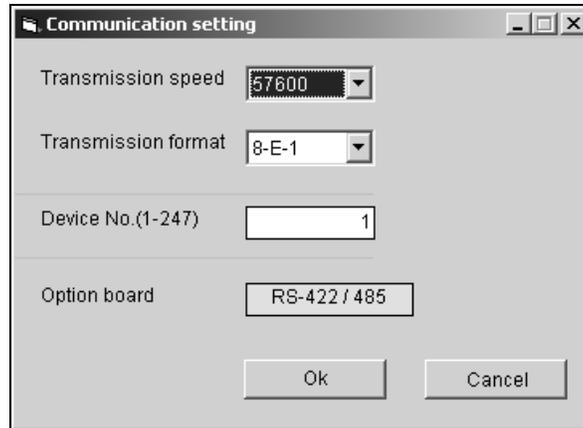
The window displays the type of Serial Communications option module that is installed on Port 2 of the MicroMotion Module.
