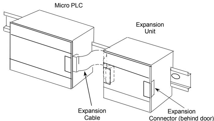
The Micro PLC and MicroMotion Module(s) must be connected in the same orientation. Connecting any expansion unit “upside down” will damage the DC input circuit when the system is powered up.
