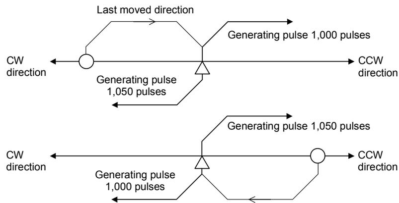
In Homing Mode, the result of Backlash Compensation depends on the travel direction and the type of homing being performed.
