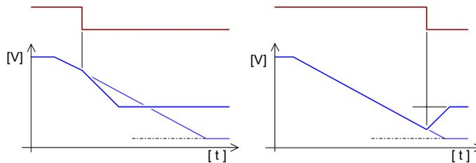
**Feedrate Override Percentage (Common Parameter 18):** If the Feedrate Override (FE) input is enabled (above), specify a constant percentage by which to decelerate the pulse rate when the external FE input turns On. This defaults to 100%, which causes the pulse to stop immediately. The pulse will not slow down below the initial velocity, even if a slower speed is specified.
