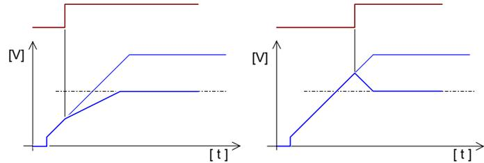
*FE Input OFF when Accelerating during Feedrate Override*
