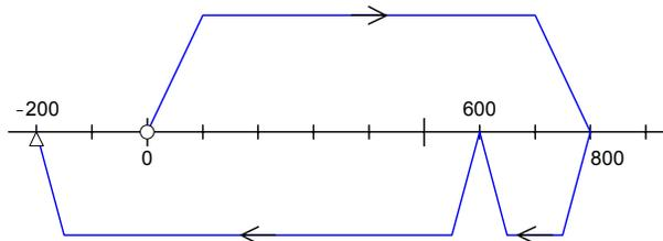
**Absolute + Incremental Target Positioning for Linear Moves**
