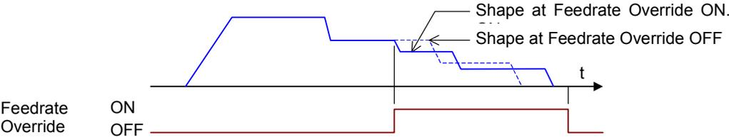
If Feedrate Override is turned Off before the end of the operation, the speed returns to its former rate.
