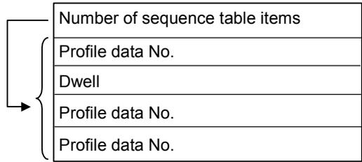
In the Sequence Table, each profile or dwell is represented as a number, which is the hexadecimal value equivalent to the bits in the profile or dwell. The format of the bits in the profile or dwell is shown on the next page.
