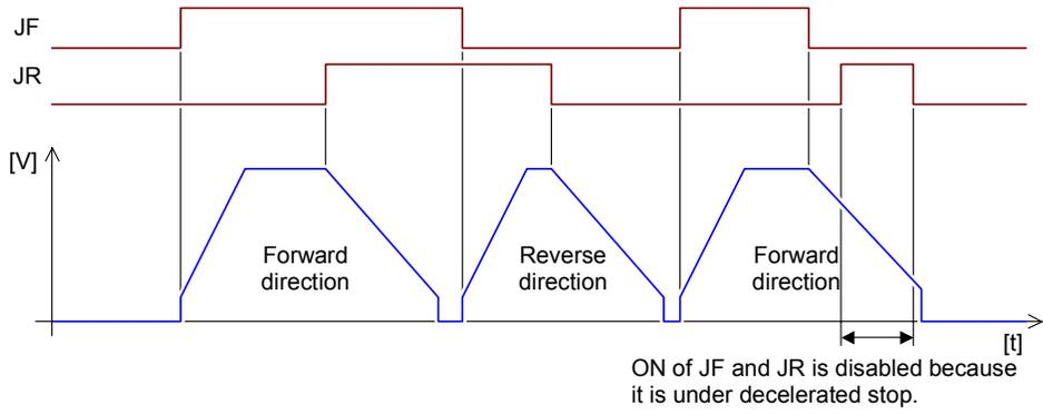
The Jog Forward and Jog Reverse inputs are level-sensitive. However, if the MicroMotion Module switches to Manual Mode from a different mode, the pulse is not output unless Jog Forward or Jog Reverse is turned Off once.
