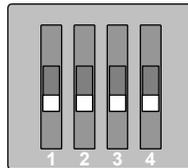
Switch 3 must be set to On to enable use of the Memory Pack for reading data in the MicroMotion module.
