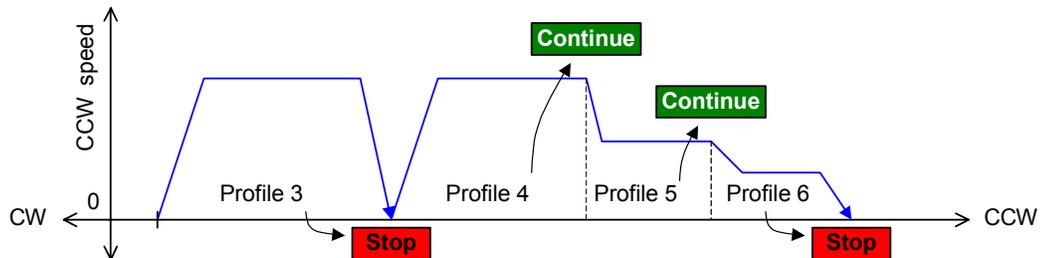
**Acceleration:** Set the Acceleration type to Linear or S-Curve.
