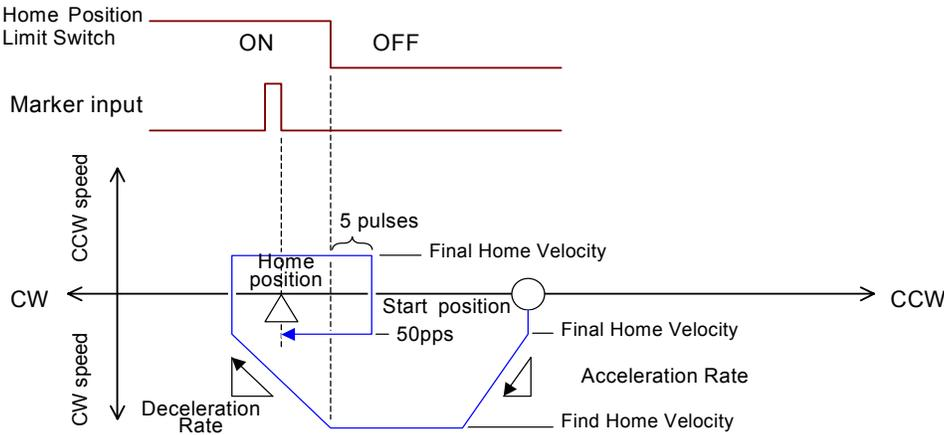
***If the Home Position Limit Switch was On at the start of High-Speed Homing [Marker Pulse]:***
