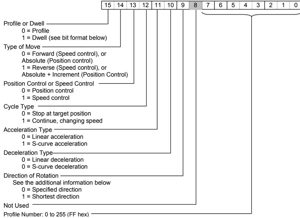
**Type of Move (bit 14):** For Position control, this bit selects Absolute or Absolute + Incremental positioning. For Speed control, this bit selects Forward or Reverse.
