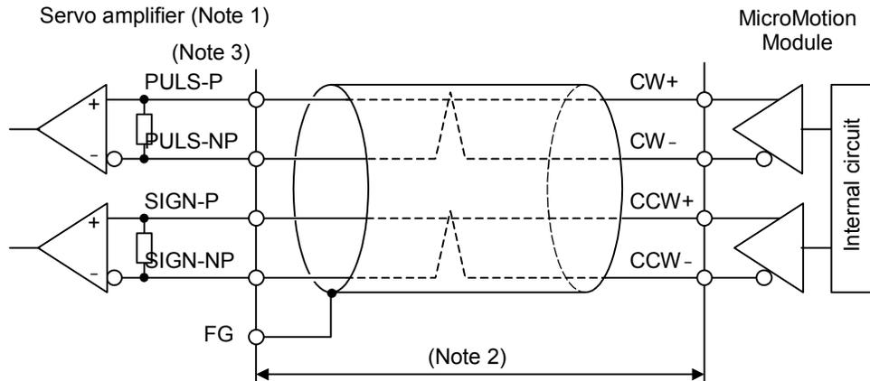
Note 1: In general, shielded cables should be grounded only on the receiving terminal side (input side). However, it may be better to leave both sides open, or to ground on the sending terminal side or on both sides, depending on the noise environment and the ground conditions.
