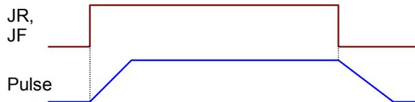
In Inching mode, if the Jog Forward or Jog Reverse input is on, a pulse that corresponds to distance that user set is output at the Initial Velocity that has been set up for Manual Mode.
