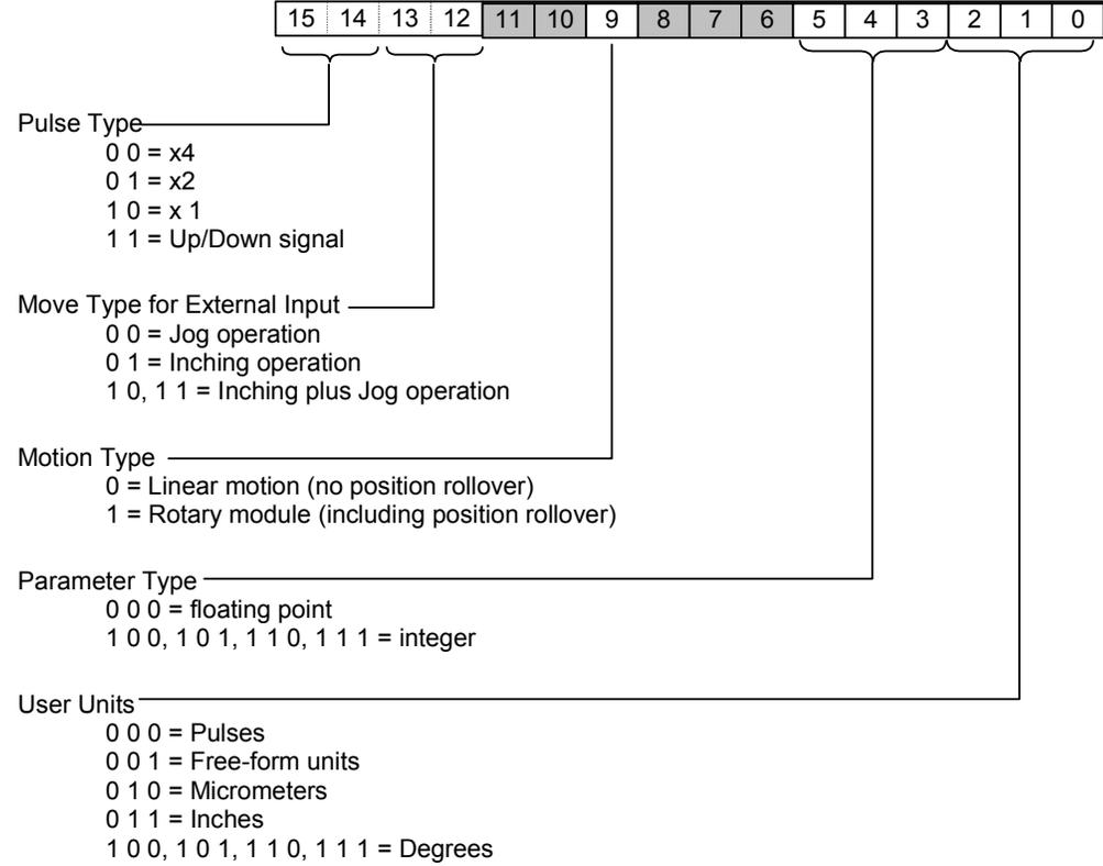
**Holding Registers 102, 202: Common Parameters for External Inputs**
