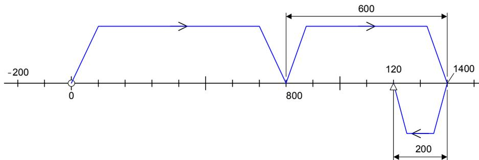
**Absolute Positioning for Rotary Moves**
