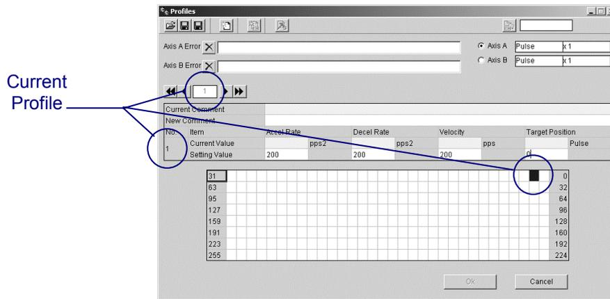
In the graphic display, edited profile numbers are represented in dark blue. Profiles saved in the Motion Expansion Module memory are represented in cyan.
