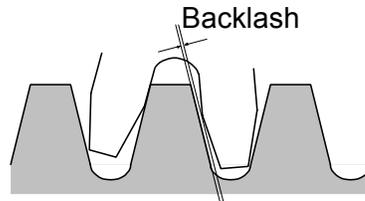
For example, if the target position data is 1,000 pulses / -1,000 pulse, and the Backlash Compensation is 50:
