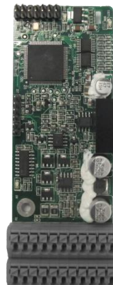
Resolver PG card AS28ENC0002
