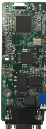
PROFIBUS-DP communication card AS28PBS0001
