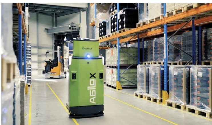
🔍 Robot AMR marki Agilox do transportu palet z detalami
