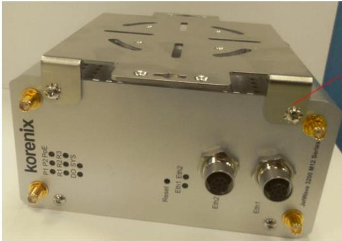
**Unlock the original screws, then lock the attached screws.**
