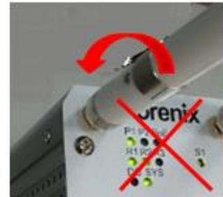
**For vibration environment**, we don't recommend you connect the antenna directly to the device, no matter how heavy you lock it. It is suggested you install the antenna at non-vibration or low vibration place and connect it by extended Radio cable antenna to the device.
