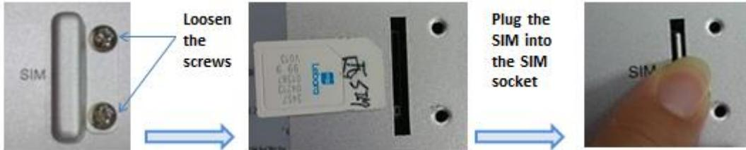
The supported SIM card is standard SIM card. If your ISP provide you Micro-SIM or Nano-SIM, please find the SIM card format carry board for the SIM socket.
